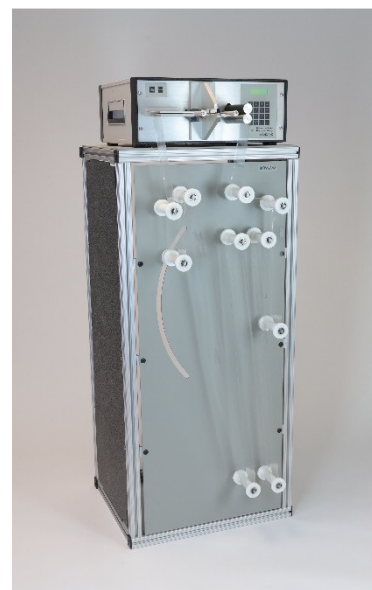
Gauge Stand shown with CX-1000 Film Thickness Gauge and 18 ft – 8 inch Polyester Film Sample inserted in stand accumulator
